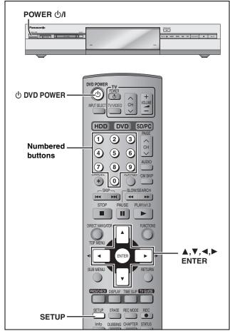
After plugging the unit into your household AC outlet and pressing [<sup>(</sup>⊕ DVD POWER] to turn the unit on for the first time, the unit starts TV Guide On Screen<sup>™</sup> system setup.
